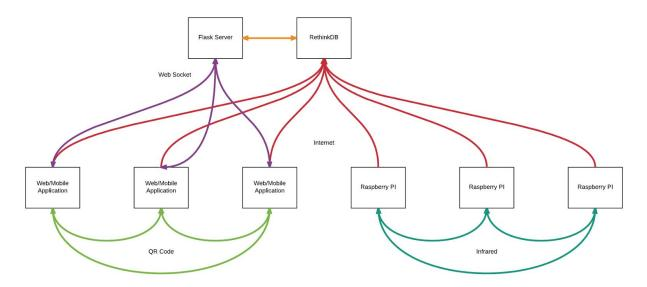
In short the system has: Flask Server, RethinkDB, web client, and Raspberry PI. Flask Server is used to serve the web client as well as to communicate the RethinkDB to all web client via Web Socket. RethinkDB is the database chosen for this project. The sociometric clients are all the Raspberry PIs and web clients connected into the RethinkDB. The web client serve two purposes: to display the real time data as well as mobile-ready implementation of the alternative to the Sociometric Badge.
